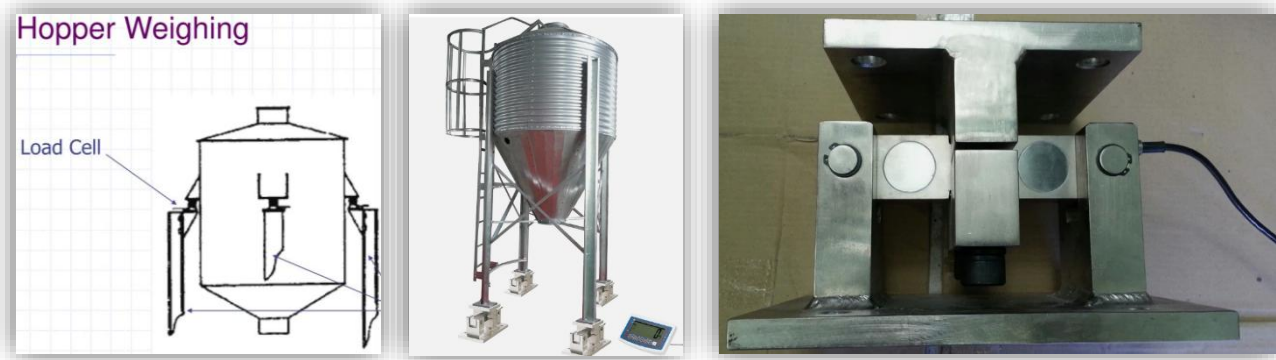
Figure 9: Hopper silo weighing system.
